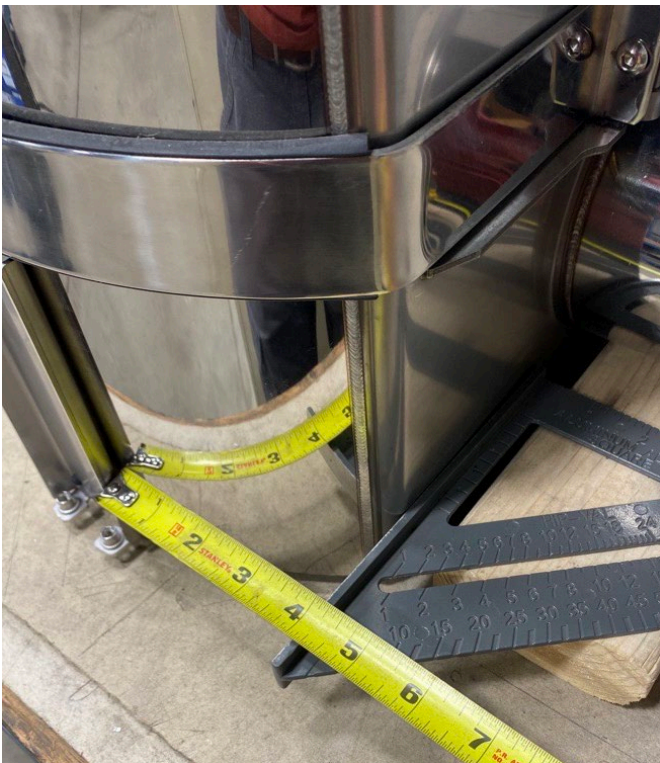
Figure 7: Measuring Rear Bracket Position (Driver Side)
