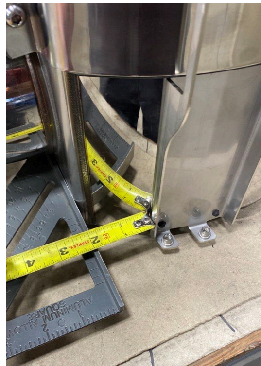
Figure 8: Measuring Front Bracket Position (Driver Side)
