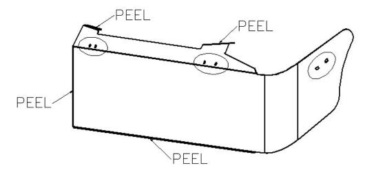
Figure 3: Flanges & Holes to Remove Protective Plastic From (driver side shown)
