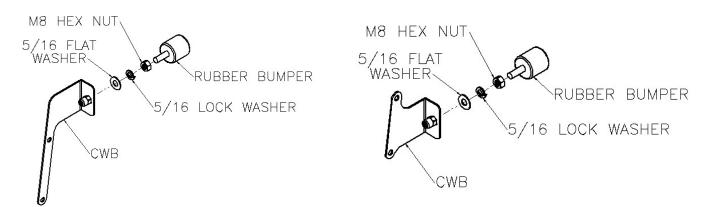
Figure 2: Rubber Bumper Assembly (CWB Shown) (PNL20731027CWB on the left & PNL20731028CWB on the right)
