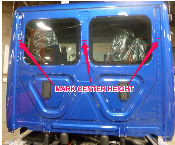
Figure 1 – Marking Center Lines
