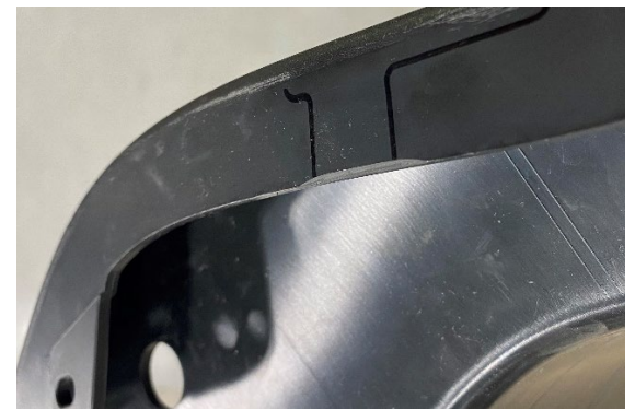
Fig 2: Chamfer Needed for OEM Mid Roof Panels
