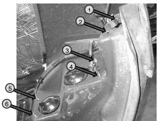
Figure 4 Headlight/Signal Nuts
