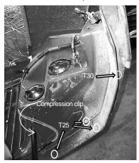
Figure 5 Headlight/Signal Torx fasteners & clip
