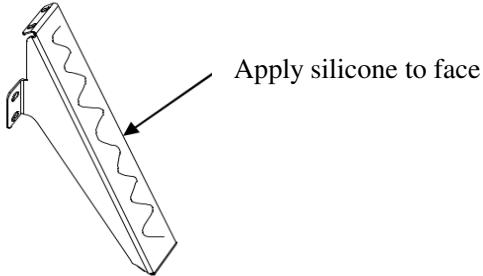
8. Using the supplied 1/4-20 x 1" hex head bolts, washers and lockwashers, loosely install the brackets to the roof.
