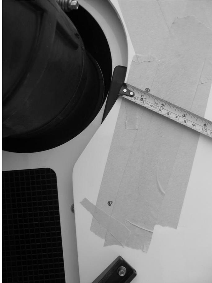
*Using your fingers, feel around the back (inside) of this location prior to drilling to ensure that your marked location is still outside this rib. If your marked location is not outside this rib, you may not have access to the bolt to install a nut on the back side after you drill the hole. As a guideline, this hole should be 1-1/16" from the circular edge of the hood.*
