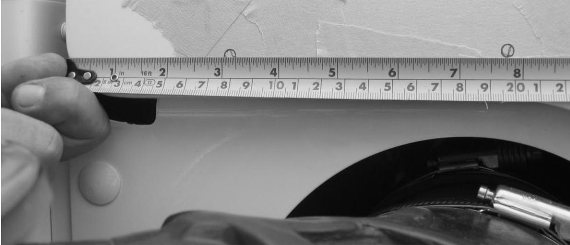
Measure and mark the horizontal placement of these holes on the previously mentioned centerline. The first hole will be located at 3-1/8" from the rear edge of the hood, while the second will be located at 7-3/4" from the rear edge of the hood.
