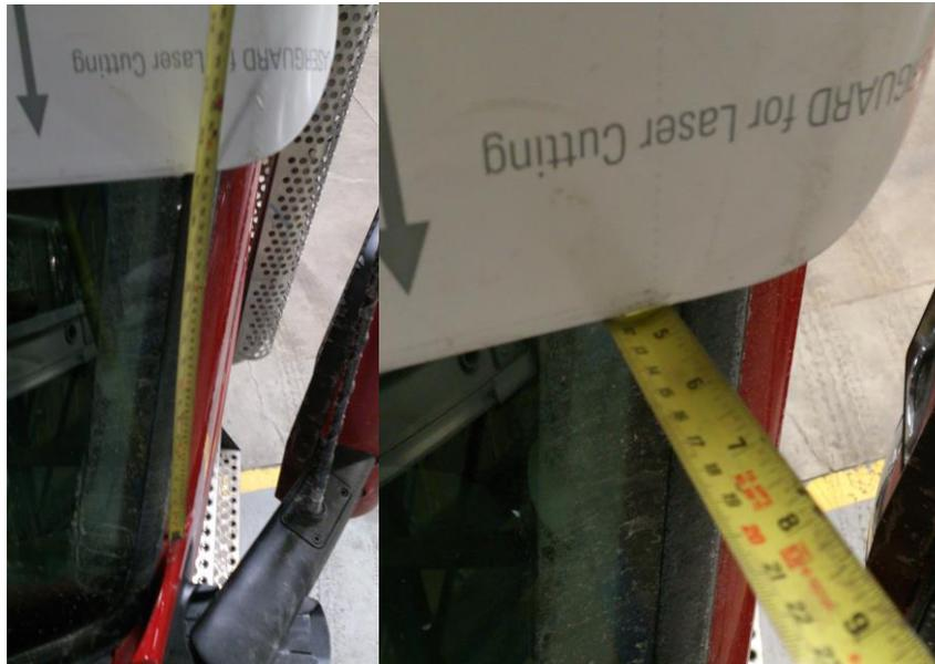
13. Using a pen, mark the hole centers of the outside bracket holes on the taped section and the two end holes of the visor halves to the section above the door.
