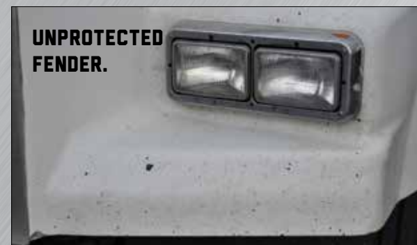
REAL WORLD SAMPLES AFTER 4 WEEKS IN SALT BATH
