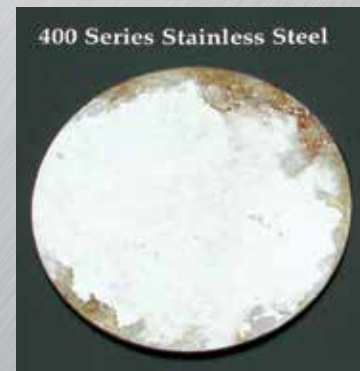
REAL WORLD SAMPLES AFTER 4 WEEKS IN SALT BATH
