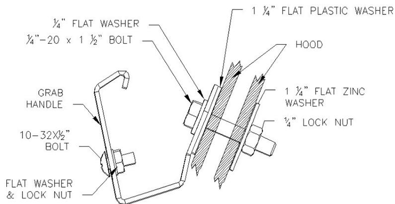
10. Peel plastic from around the Grab Handle mounting holes and five mounting slots from the Surround top section.
