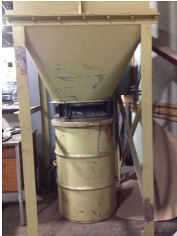
Figure 3. Pictures of Dust collector system that capture laser dust.
