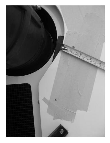
Using your fingers, feel around the back (inside) of this location prior to drilling to ensure that your marked location is still outside this rib. If your marked location is not outside this rib, you may not have access to the bolt to install a nut on the back side after you drill the hole. As a guideline, this hole should be 1-1/16" from the circular edge of the hood.
