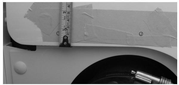
The two horizontal mounting holes should be marked on a shared horizontal centerline, <sup>3</sup>/<sub>4</sub>" from the edge of the hood above the intake boot as shown above.
