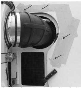
Four mounting hole locations are required as shown in the picture above.
