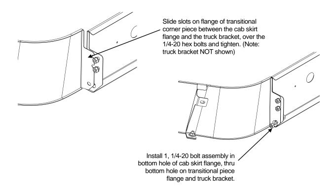
12. Clamp transitional corner piece to sleeper skirt. Once fit is established, bolt corner skirt to sleeper skirt using 1/4-20 hex head bolts, flat washers and hex lock nuts supplied.
