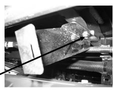
Replace with bracket supplied in kit. Fasten using clips and bolts
