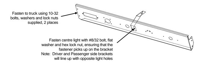
10. Loosely bolt sleeper skirt to truck using clips and bolts removed in step #1. \*Newer models will use Carriage Bolts with provided retaining washer, 5/16" flat washer, 1/4" flat washer and Nylock Nuts
