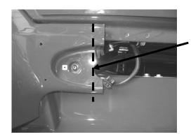
15. It is necessary to cut away part of the factory panel at the front of the cab. Cut at edge of light hole, as shown. Reinstall the front piece of the factory cab skirt and the hood latch hook.
