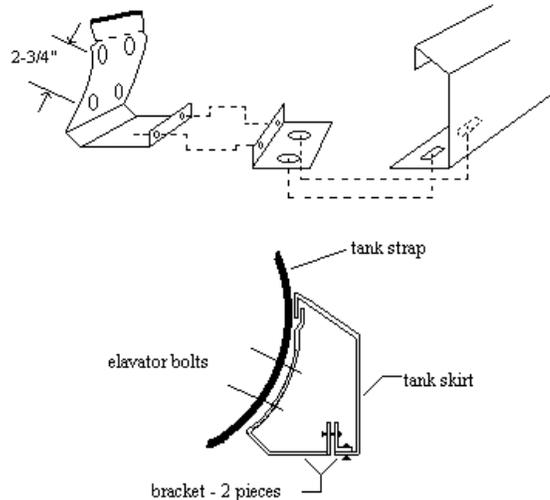
6. Insert elevator bolts through backside.
