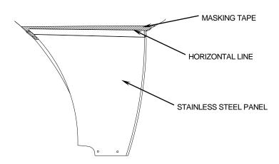
3. Remove panel and place bracket over the offset bend of hood, 1/16" below the horizontal line on the masking tape. Mark and drill 6, #11 holes into the hood. Remove masking tape and fasten the bracket using the pop rivets supplied.
