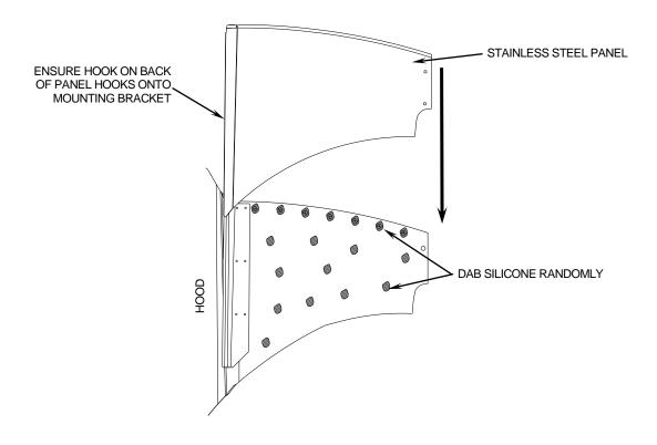
7. Close the hood and drill 2, 1/4" hole through bottom square holes into hood. Slide spacer washers between hood and panel. Install 1/4-20 carriage bolts through holes and secure using 1/4 flat washers and 1/4-20 lock nuts supplied.
