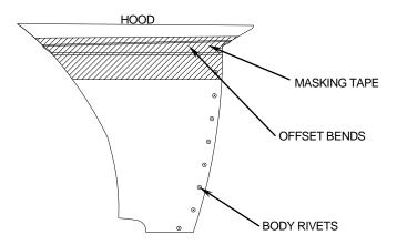
2. Remove plastic coating from hem of panel and from around the bolt holes. Place stainless steel hood panel on the hood and mark a horizontal line along the top edge of the panel onto masking tape.
